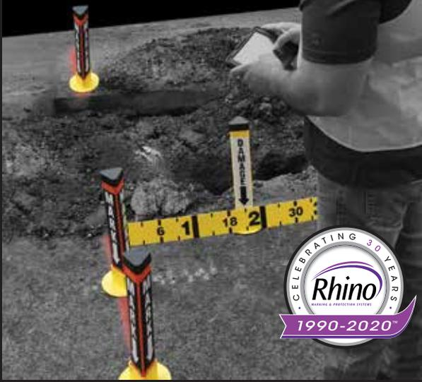
The Rhino HIT Kit +2 is the recognized industry-standard damage investigation tool. It provides posts that are legible from 360° and includes a rigid ruler with numbers that can be clearly read from a distance. [RhinoHitKit.com](http://RhinoHitKit.com) | 800.522.4343
