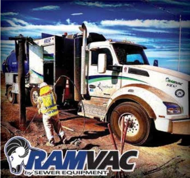
RAMVAC offers air and hydro excavators with vacuum power from 1400-5400 CFM @ 18-28" Hg and debris body capacities from 2-15 cubic yards. Non-CDL options are available, as well as rental, rent-to-own and preowned units. With nationwide service locations and a parts/accessories online store, RAMVAC has the solution for your vacuum excavation needs.
