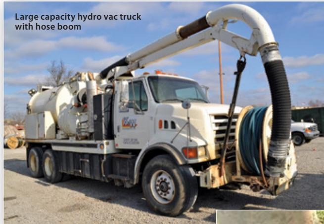
Large capacity hydro vac truck with hose boom
