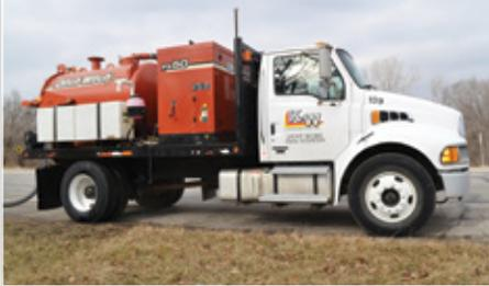
in sandy or loose type soils, but are less effective in hard clay soils or frozen ground. These air-vac systems are comprised of a high-pressure air pump with a small hose and an air lance (wand) with a nozzle designed to cut and pulverize the soil as much as possible. The results are then sucked through a large hose, typically 3-12" in diameter, then into a large tank. After the pothole is complete and ready for restoration, a large door on the back of the tank can be opened and the tank tilted
