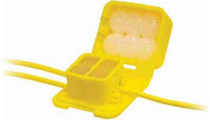
The DryConn® IDC makes waterproof tracer wire splices without the need for stripping wires! The connector's unique design allows for a service line to be installed without cutting the main line. Now the insulation displacement technology has made installation even easier by allowing connections to be made without stripping the conductor. Waterproof and corrosion proof, 50V, #14 – 12 Solid/Stranded Copper, Steel Core Tracer Wire, CCS.
